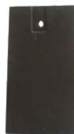
Re-Bonded Magnesia Chrome Brick
